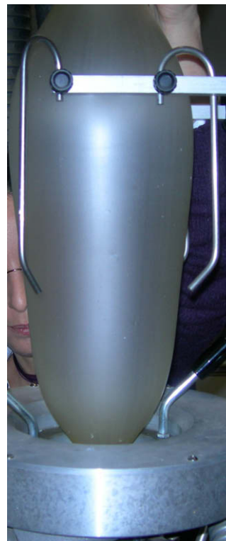
Fig. 9. Film blowing of urea/formamide thermoplastic starch (TPS 8).
